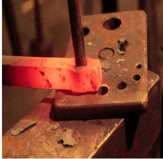
Punching a forged metal.
