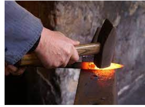
Drawing a forged metal.
